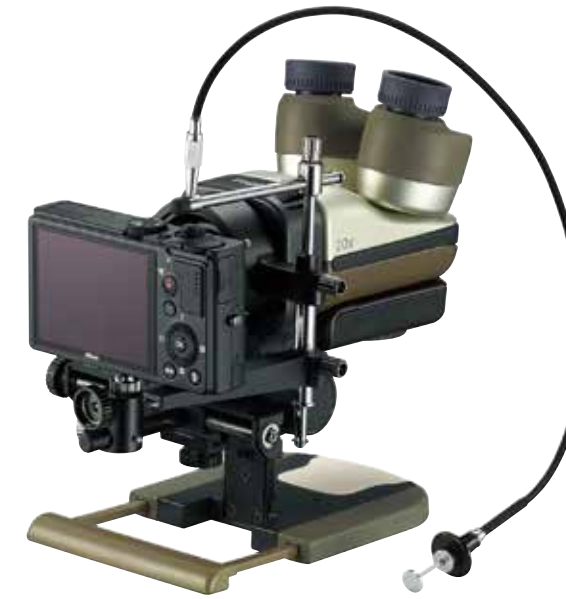
EZ-Micro + FSB-UC + COOLPIX Digital Camera
