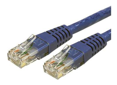
The C6PATCH100BL Cat 6 Patch Cable (100 ft) meets or exceeds all Category 6 cable specifications to ensure reliable Gigabit network connections, and features a durable blue PVC jacket that enables you to color code your network cable runs as needed.
